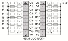
(\*) Contact CLOSED: RUN, Contact OPEN during RUN: HOLD
